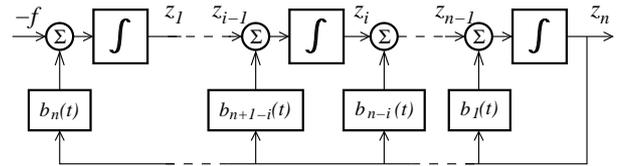
Fig. 5. The series realization represents the adjoint system.
