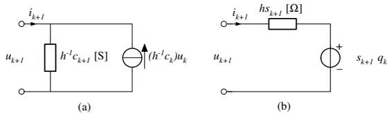
Fig. 2. Time-discrete LTV capacitor (Backward Euler). Voltage controlled (a) and charge controlled (b).
