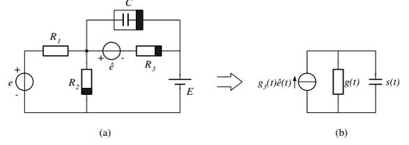
Fig. 1. Original nonlinear circuit  $\mathcal{C}$  (a) and reduced LTV small-signal circuit, with  $g = G_1 + g_2 + g_3$  (b).
